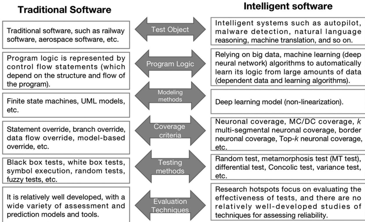
Figure 5. Comparison of traditional and intelligent software.
