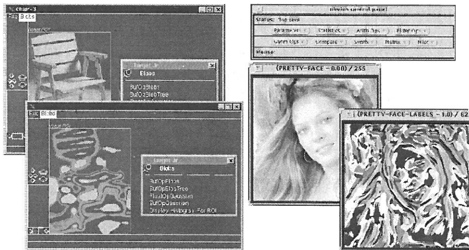
Fig. 12. (a) The blobs system uses Interviews for GUI and the class library TargetJr, the code is written in C++. (b) The local structure segmentation as implemented using: a LispView GUI, Obvious process control. The actual segmentation code was written in Common Lisp.
