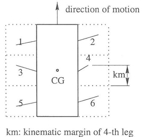
Fig. 1. A schematic diagram of a six-legged robot.
