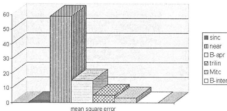
Fig. 4. Six different reconstructions: reconstruction with sinc, nearest neighbor, 3-rd order B-spline approximation, linear interpolation, Mitchell reconstruction with  $B = C = 1/3$  and 3-rd order B-spline interpolation.
